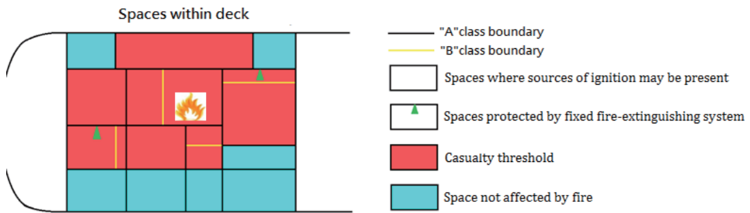
Figure 1.5.2(2)b Not protected by fixed fire-extinguishing system
